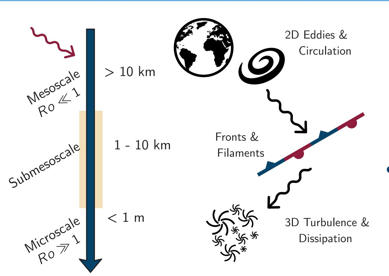
**Front:** A region with a large horizontal buoyancy gradient,  $M^2 \equiv \partial_x \bar{b}$ , typically in near-geostrophic balance.
