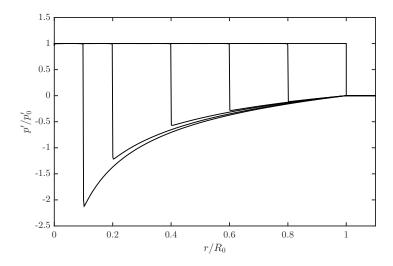
Figure 2: Nondimensional pressure anomaly for the relaxation of an isochorically heated cylindrical jet. Shown here (from right to left) at t = 0, 0.2, 0.4, 0.6, 0.8, & 0.9.
