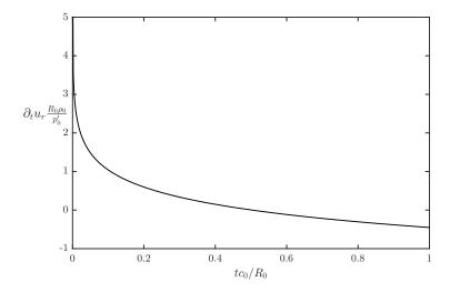
Figure 4: Nondimensional outward radial acceleration of the cylindrical jet surface in time, from t = 0 to the singular point at t = 1.
