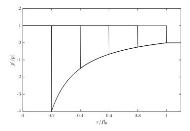
Figure 1: Nondimensional pressure anomaly for the relaxation of an isochorically heated spherical drop. Shown here (from right to left) at t = 0, 0.2, 0.4, 0.6, & 0.8.
