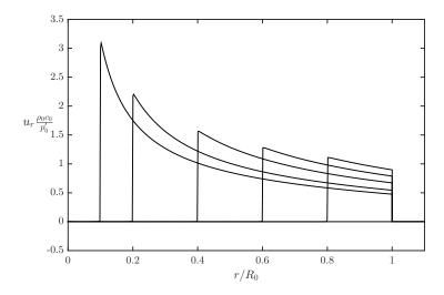
Figure 3: Nondimensional radial velocity profile for the relaxation of an isochorically heated cylindrical jet. Shown here (from right to left) at t = 0, 0.2, 0.4, 0.6, 0.8, & 0.9.
